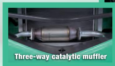
Three-way catalytic muffler
