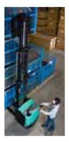
AC (alternating current) drive motors have given these pedestrian stackers a number of added advantages – including higher economy, energy efficiency and power. An ergonomic tiller arm and extremely compact powerhead, combined with a very narrow chassis and excellent visibility, makes them highly manoeuvrable in even the smallest of spaces. They can be used, for example, on board road vehicles, in block stacking or in congested areas.
