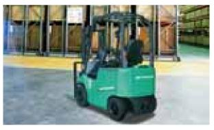
Whether you choose 3 wheels or 4 wheels, the same advanced engineering applies. We have 4 wheel pneumatic tyre electric counterbalance trucks at capacities of 1.0 to 2.8 ton and 3.0 ton, as well as cushion tyre models at capacities from 1.5 to 5.5 ton.
